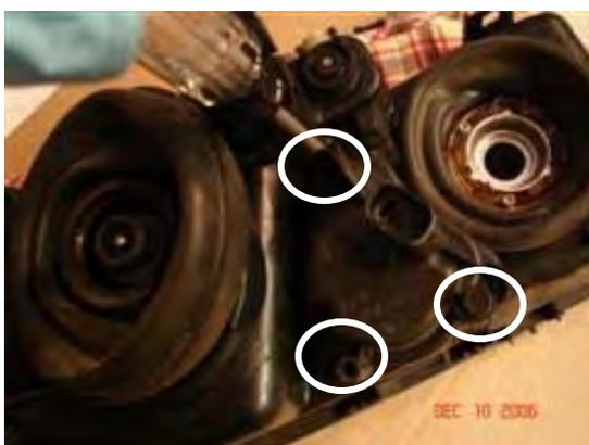
Remove the 3 screws holding the Height adjuster motor. At the end of the shaft is a ball that slides into a track on the back of the inner headlight assembly. **DO NOT PULL THIS STRAIGHT OUT.** You need to push in and slide the ball to the right to remove. You are essentially working blind. It took me an hour to figure this move out!
