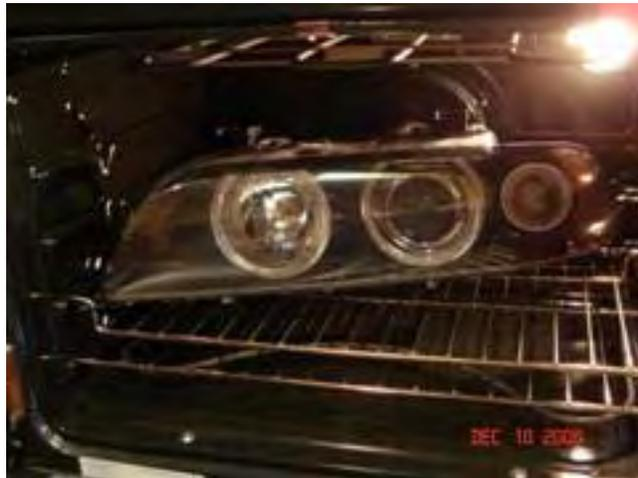
Start at one end with a screwdriver or flat blade and separate the clear front cover from the main body. You will need to lift the clear tabs over their holding post as you go. You will see the “black” goop start to give up its hold. Take your time and go a little at a time. Work your way around the entire lens.
