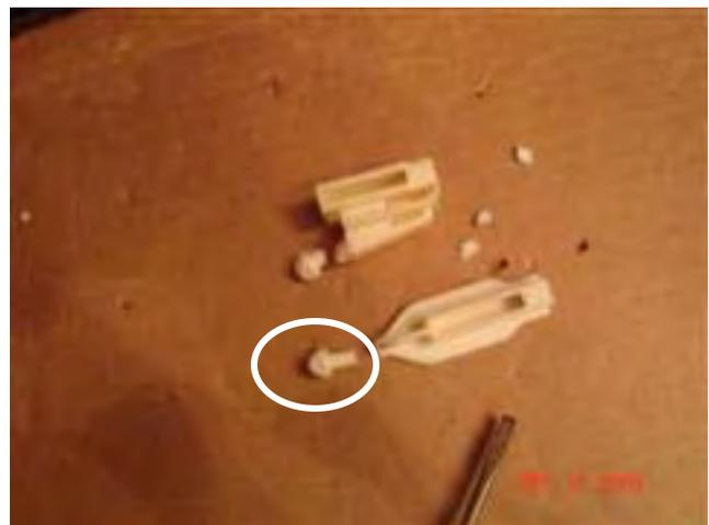
**Pop the light assembly into the new pieces and reverse the disassembly order. Use the oven to heat up the lens and body to “glue” the two pieces together. Go out and enjoy your new headlights.**
