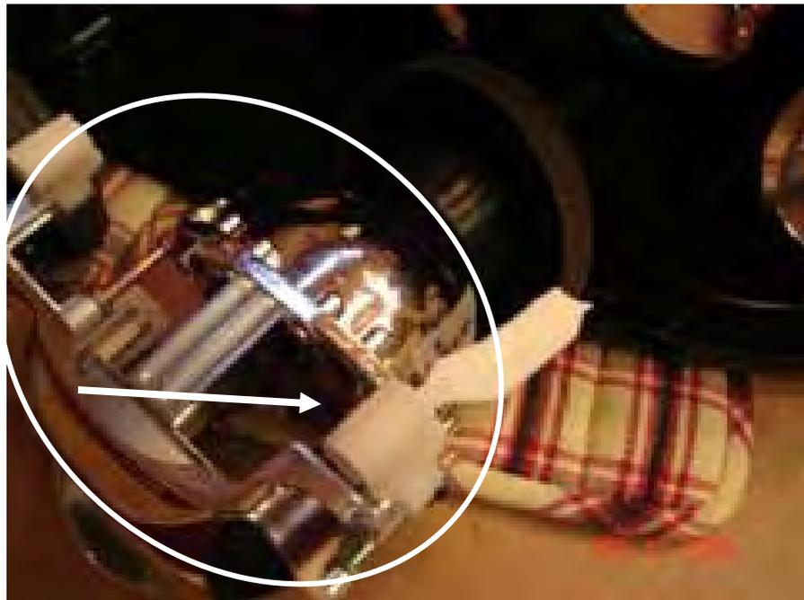
Broken piece on chassis. Use the adjuster on the back side to turn the screw to release what left of the original piece.
