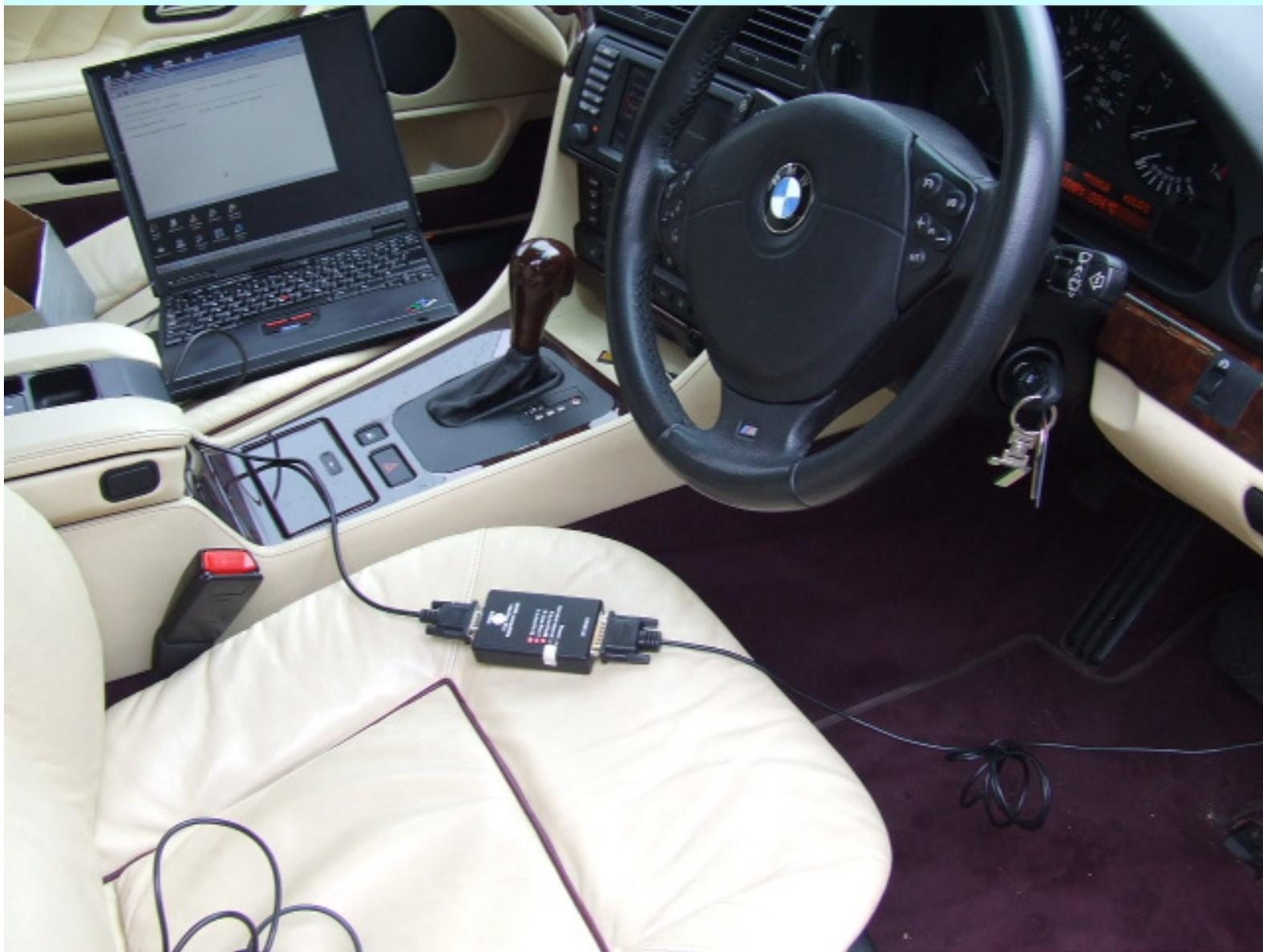
The internal OBDII connector is used for testing the DME (engine control unit) and EGS (transmission control unit) only, you will not be able to test any other module from this connection.
