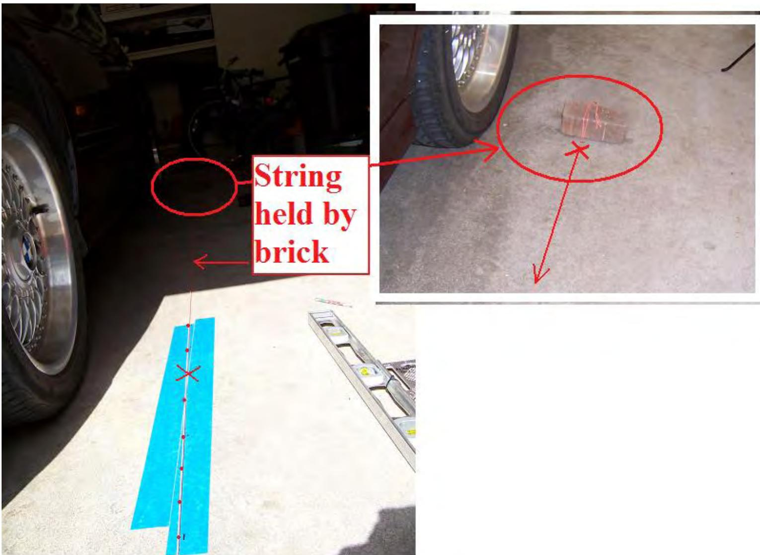
7. Now measure Camber. I have calibrated my device so when the bubble is barely out of the marks, it is roughly 0.50 degrees (or 30 minutes, which is half of a degree). In fact this is  $-0.50$  degrees, so it was good:
