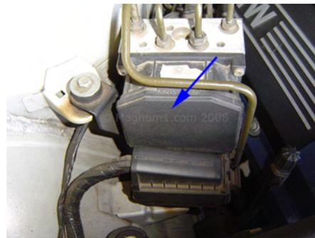
Take your screwdriver and carefully pry open the lock on the plug, like so, now grasp the plug and pull it off:
