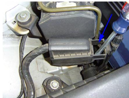
Then remove the 6 torx head bolts, again 3 on each side, the bottom left and right are the most difficult to get at:
