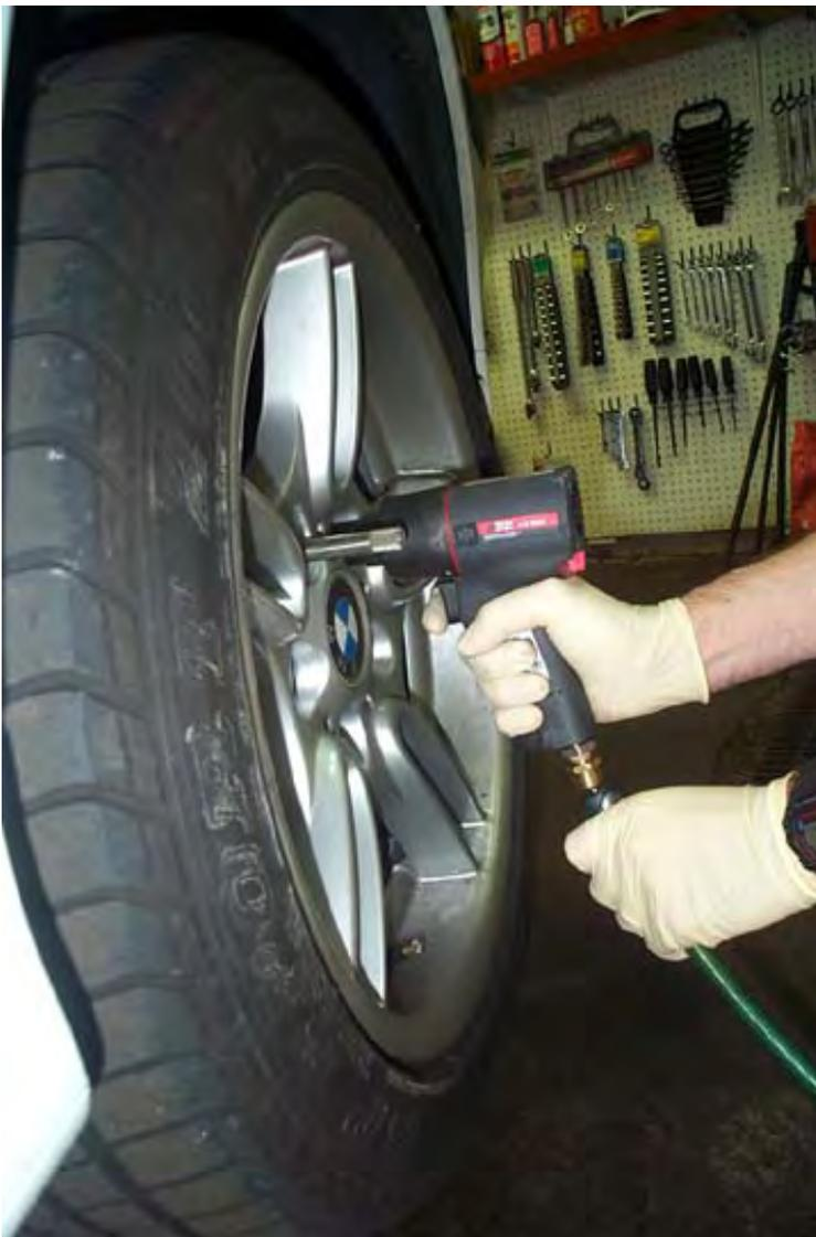
Remove the rear wheels using a 17mm 6-point socket.
