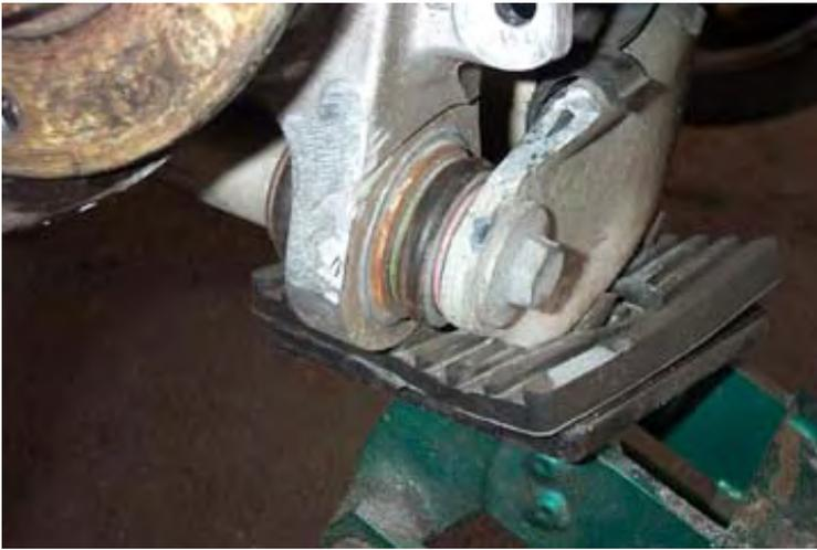
Right next to the part of the control arm you are about to grind is a rubber boot. It is very easy to nick this boot with the angle grinder. You don't want to do this, since taking that part of the suspension apart in order to install a replacement boot is not easy. So how do we protect the boot?
