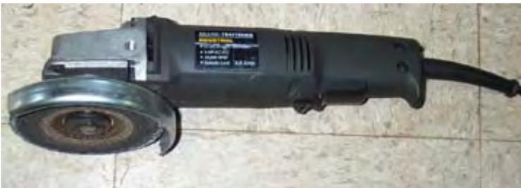
For the next few steps, you'll need an angle grinder such as the 4 1/2" Sears model shown here. It will be used to remove material from the control arm and knuckle.
