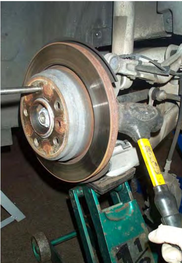
Check that the parking brake is **not** engaged.
