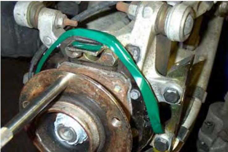
Reattach the backing plate with the four 10mm bolts. Install the modified support bracket with two 16mm bolts. Reinstall the rubber gasket.
