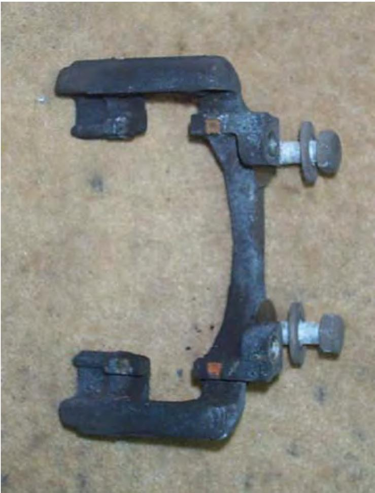
Use a 16mm socket to remove the two bolts holding the caliper frame.
