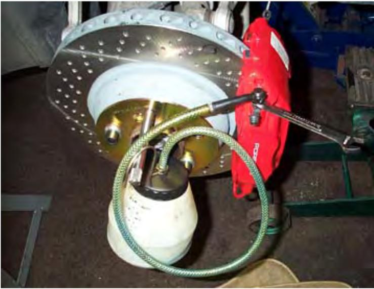
Place an 11mm 6-point box end wrench over the outer bleed screw. Attach the hose from the brake fluid catch bottle to the nipple on the end of the bleeder screw and crack open the screw about 1/4 turn. If you are using the pressure bleeder, leave the screw open until the large air bubbles stop coming out and mostly fluid is visible through the clear hose. Tighten bleeder screw and repeat process on the inner bleed screw.
