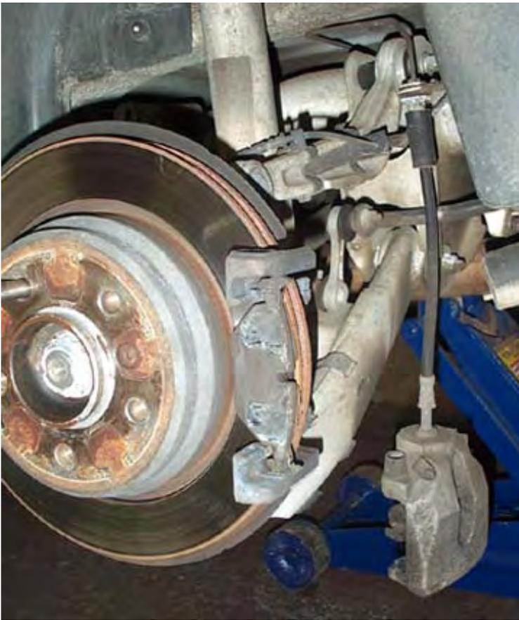
Wiggle the caliper until it pulls off the rotor. The outer pad will remain behind on the frame, while the inner pad will stay clipped to the caliper. Don't force anything. It should come off after a bit of wiggling.
