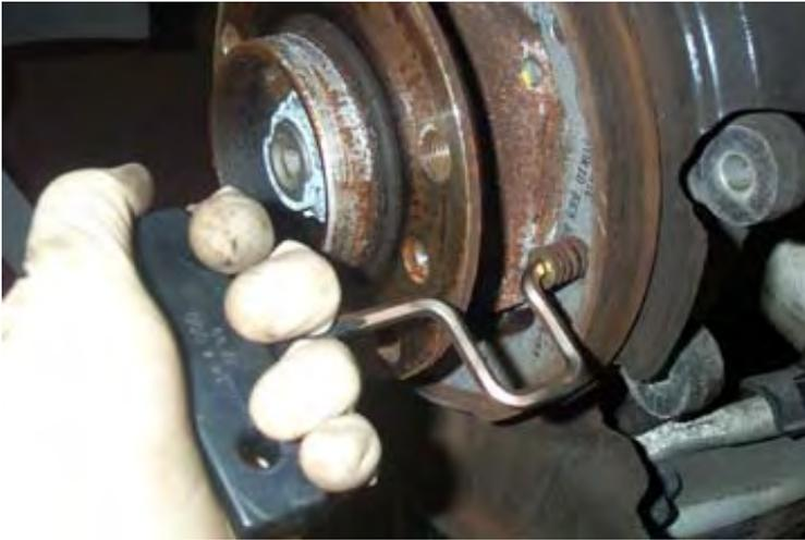
Using the special tool, attach the new parking brake shoes to what remains of the backing plate by inserting the spring loaded pins and rotating them 1/4 turn. The pins go through a hole in the shoe and then through a slot in the backing plate. If you use a flashlight from behind, it's easier to line up the pins properly.
