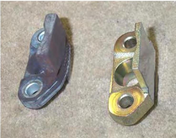
The upper support you just removed will be replaced with a new one that mov'it has machined to fit within the Porsche rotor hat. The old piece is shown on the left. The new one is on the right. (Don't install this yet.)
