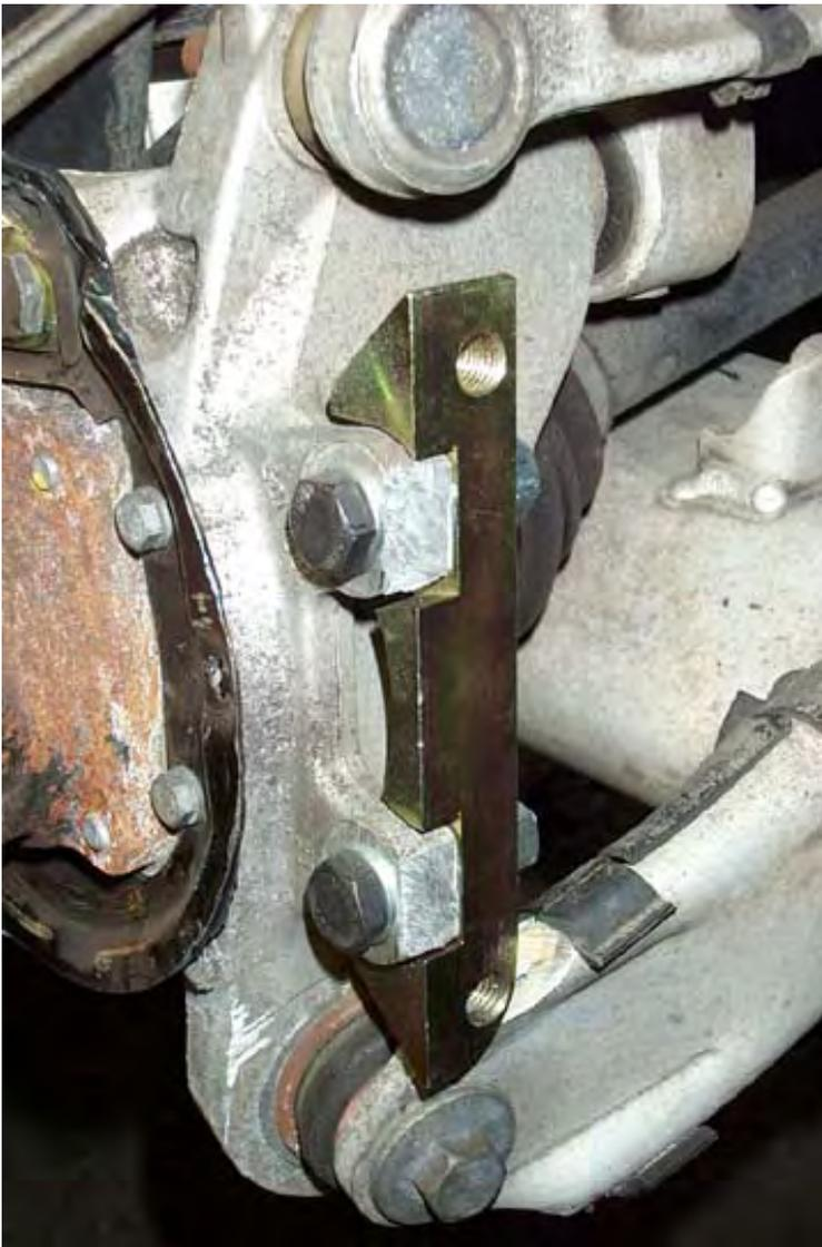
Two different thickness shims were included in the kit to move the bracket slightly toward the center of the car. At this time, you should use the thicker shims, placing one between each aluminum ear and the bracket before installing the nuts.
