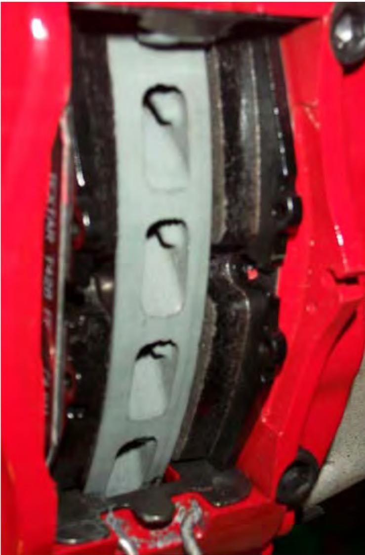
When you insert both pads, they should align fairly closely to the curvature of the rotor as shown here.
