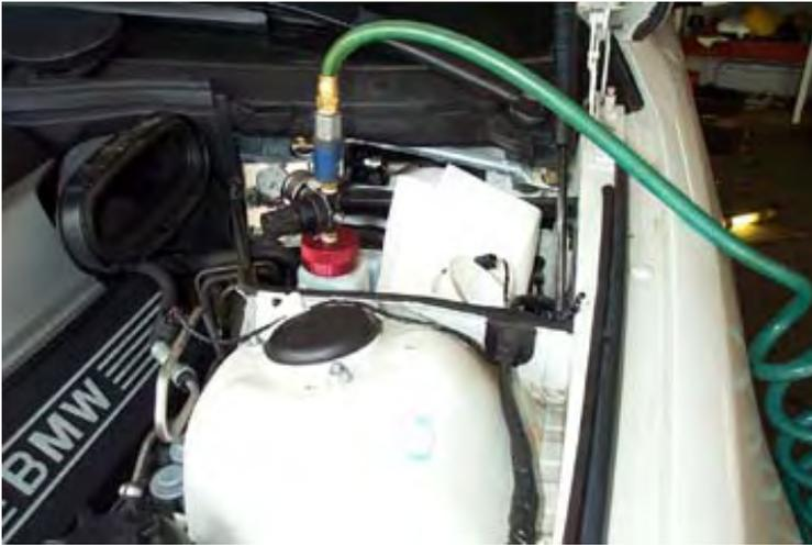
Bleeding the brakes comes next. Shown is a pressure bleeder with an adjustable pressure regulator and a built-in pressure gauge. It's possible to do this without the pressure bleeder, but this makes it easier to get a good bleed.
