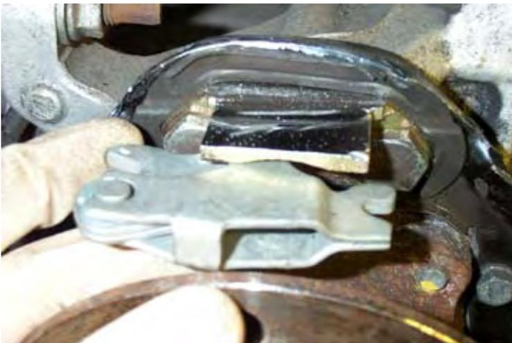
Now it's time to assemble the parking brake. Extend the end of the parking brake cable with a pair of needle nosed pliers. (You had pushed it into the hole earlier, prior to cutting the backing plate.)
