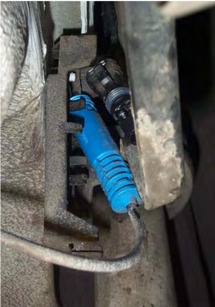
enters a small plastic holder. Both brake pad wear sensor and ABS sensor harnesses terminate here. Disconnect the brake pad wear sensor connector by squeezing the retaining tabs on the male end and pulling it straight out.
