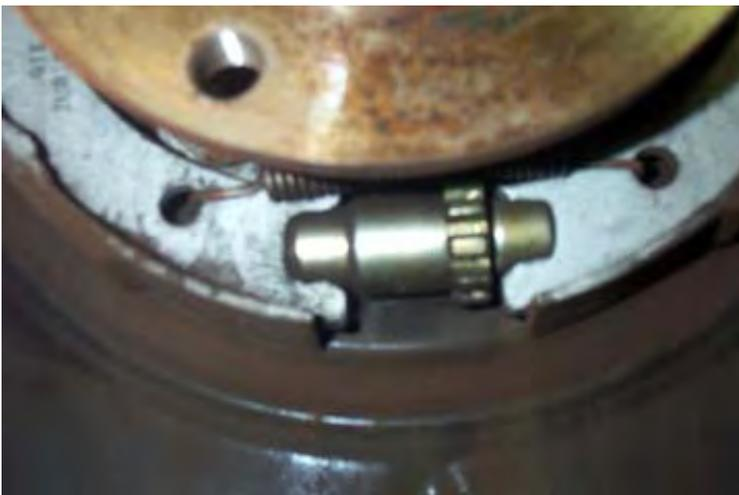
Slip the rotor over the parking brake/hub assembly and rotate it. If there are no scraping sounds, remove the rotor and turn the adjusting wheel with the tip of a screwdriver a couple turns to push the brake shoes apart. Then test fit the rotor again. Keep doing this until the shoes just barely touch the rotor. Then back off by 1/4" turn.
