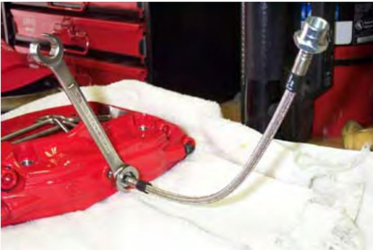
There may be a red plastic cap and rubber washer on the Porsche caliper designed to keep out moisture during shipping. If so, remove and discard the cap and washer.
