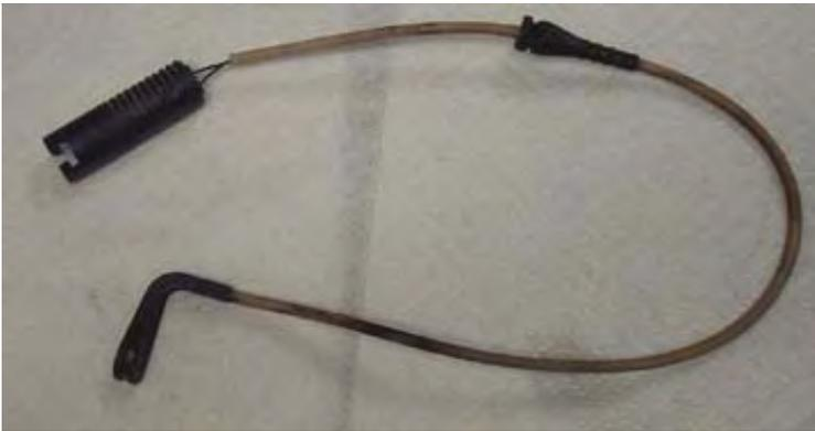
On the passenger side is a wire harness with a sensor attached to one of the brake pads. When the pad wears out, a wire is cut and a warning appears on your dash. We will disable this warning function.
