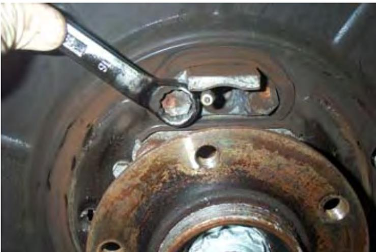
Using a 16mm offset wrench, remove the two bolts shown and pull out the upper support. Also pull out the rubber gasket that goes around the upper support. Note the orientation of the gasket. The depression faces out, as shown in the photo. It won't fit properly if you try to install it backwards in a later step.
