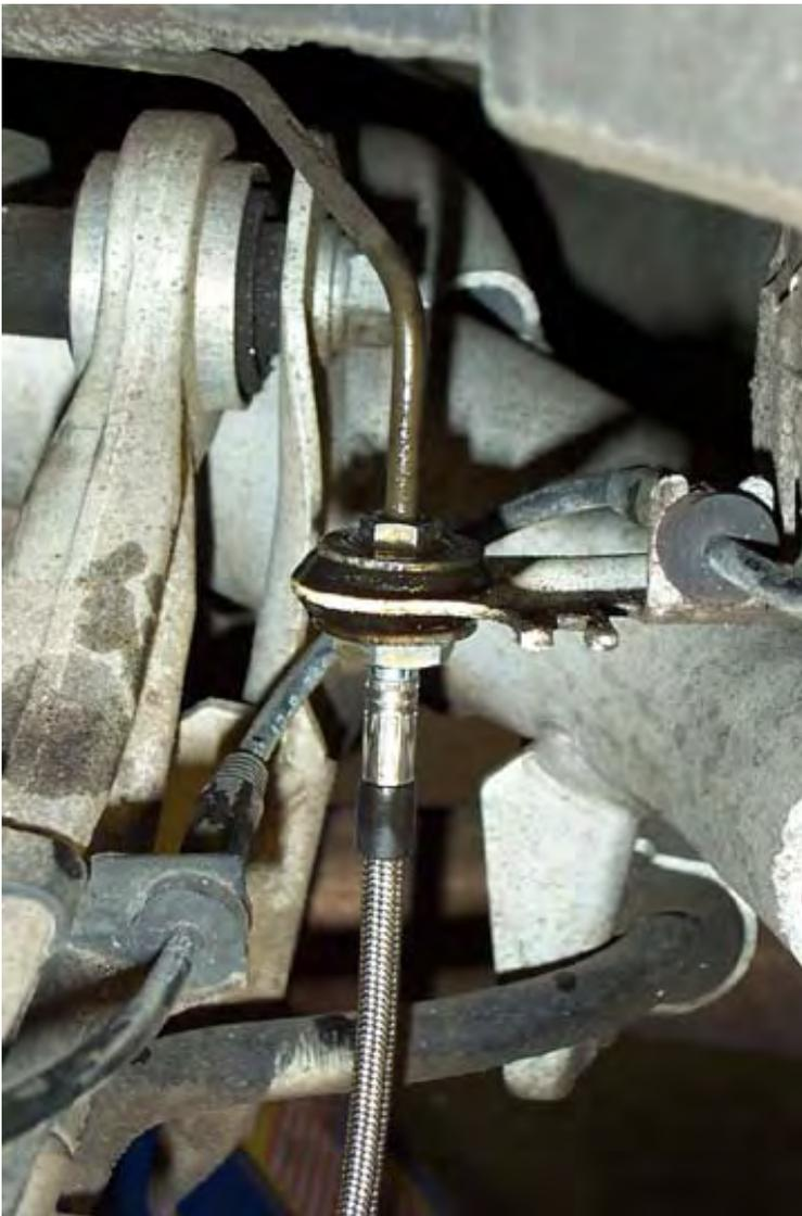
below, making sure that you reuse the original washers on either side of the grommet. Use your fingers to thread the nut properly into the fitting on the end of the flexible brake line. Tighten as far as possible with your fingers, then continue to tighten with a stubby 11mm open end wrench. At this point, you should stabilize the fitting on the flexible line with a 17mm flare wrench.
