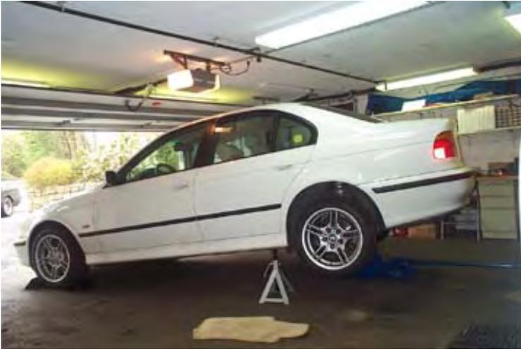
Place a floor jack underneath the differential. Jack stands go under the plastic jacking points located along the bottom of the frame rails. Lower the car onto the jack stands allowing most of the weight to rest on the stands, but leave the floor jack in place as a safety measure. Place chocks around the front wheel to keep the car from rolling in either direction.
