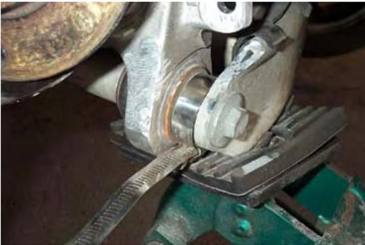
I just happened to have some hose clamps on my shelf that were the right size. Open the clamp entirely and thread the metal band around the rubber boot. Then screw it down snug enough so that the boot is compressed down out of the way and completely shielded from any careless grinder accidents.
