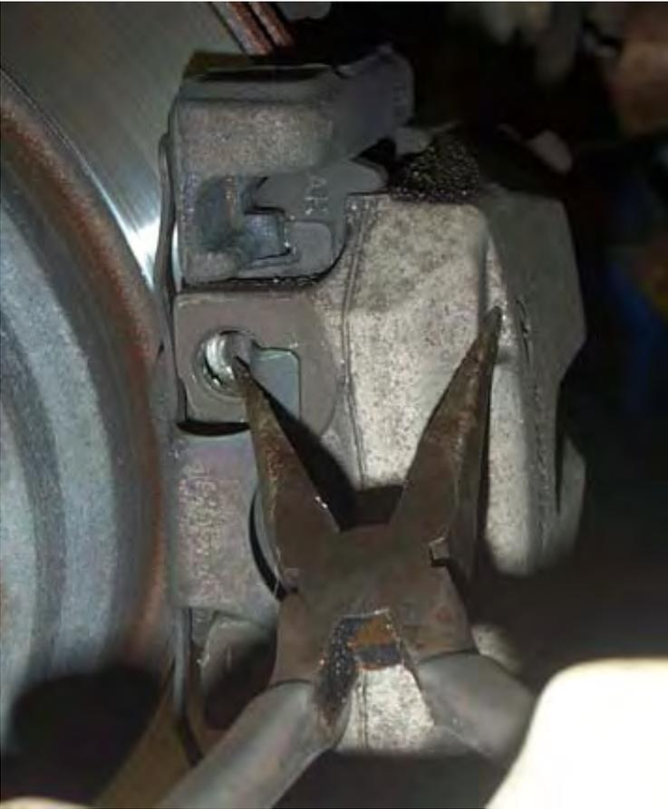
Remove the spring steel clip from the caliper.
