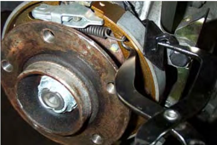
Slip the adjusting wheel into place at the bottom, between the two shoes. Then, use the brake spring pliers to reinstall the two springs. Remember, larger spring goes on top.
