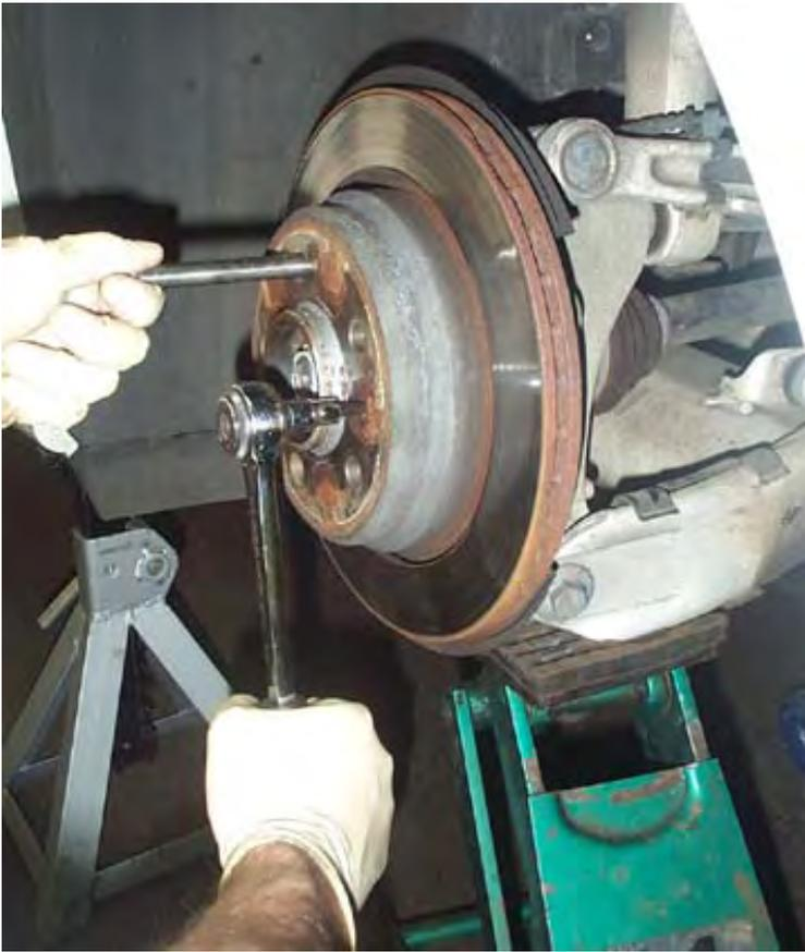
Use a 6mm Allen bit to remove the rotor retaining screw. Save this screw since you will reuse it later.
