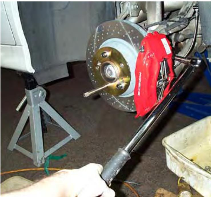
Torque the two caliper bolts to 60 Lb-ft. It's a good idea to put a small amount of blue Loctite on the bolts.
