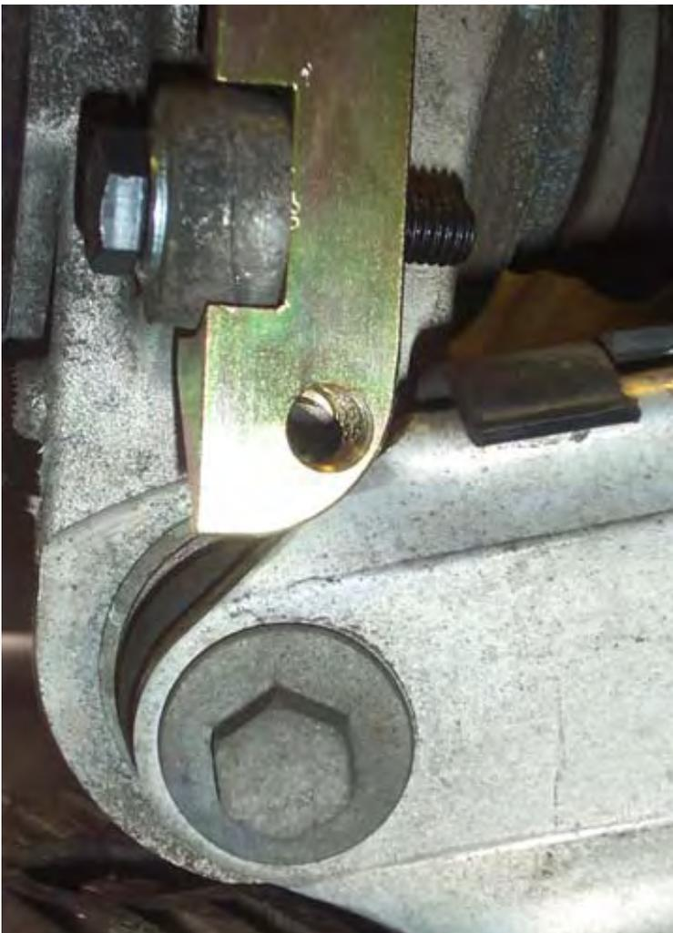
Compress the suspension with a floor jack, but stop raising it BEFORE the car lifts off the jack stands..
