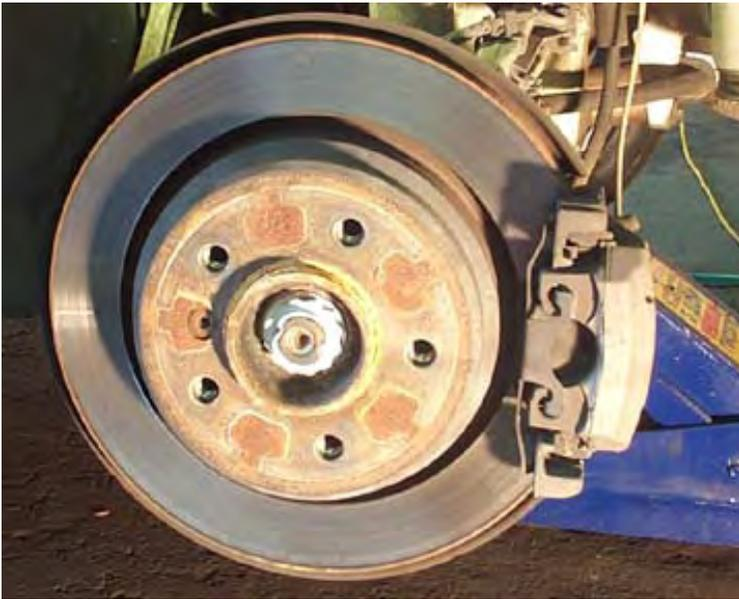
Shown is the stock 540i rear brake. Note the backing plate that extends from behind the rotor. We'll be cutting that plate to make room for the larger rotor and calipers.
