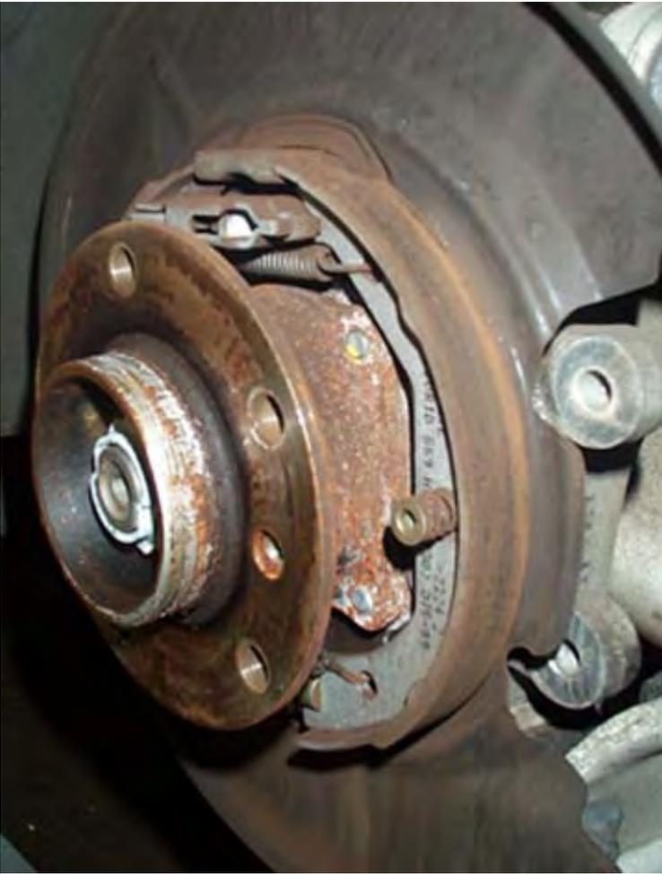
Remove the upper and lower parking brake return springs.
