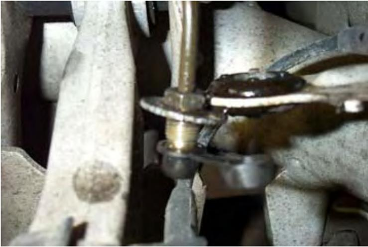
In this photo, I have pulled the hard line up and out of the bracket and rubber grommet and snapped a rubber cap on the end to stop brake fluid from leaking out. I highly recommend that you pick up such a cap at the auto parts store before removing the brake line. It prevents all the brake fluid from draining while the line is disconnected.
