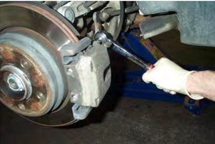
Remove the caliper from the frame by using a 7mm Allen bit to unscrew the two slide pins. The slide pins are hidden beneath plastic caps which may be pried off with your fingers. In order to get clearance for your ratchet while removing the lower caliper slide pin, you may need to jack the suspension up by placing a floor jack under the knuckle, just behind the rotor.
