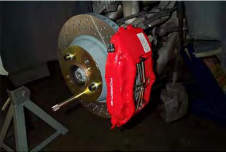
The next step is to make sure the caliper is properly centered about the rotor. Make sure there are no brake pads mounted in the caliper. Bolt the caliper to the adapter bracket using the two large allen bolts. You'll need a 10mm allen bit for your ratchet. Tighten the bolts snug enough to hold the caliper firmly in position but do not torque at this time. You will disassemble this again later.
