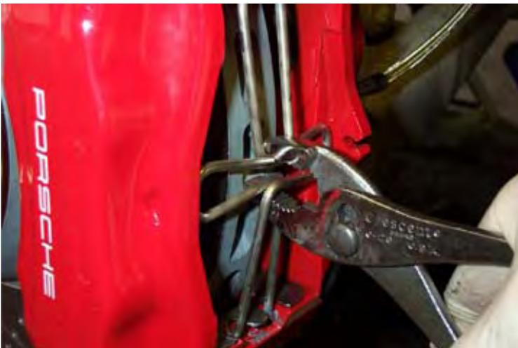
Open the pad retainer by squeezing the center together with pliers while pulling up on the end to free it from the lip that holds it down.
