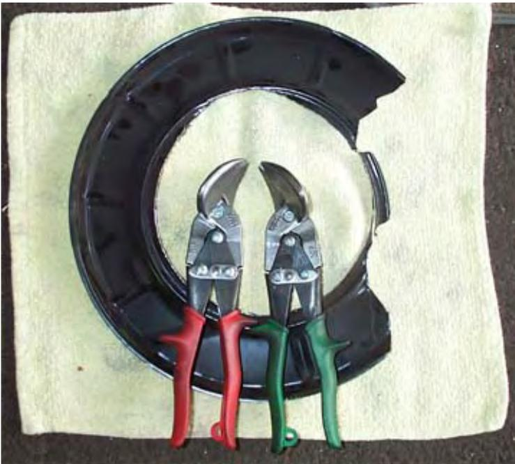
properly supported. You should cut the plate right at the point where it starts to bend, just slightly inside the score mark you made in an earlier step. Remember, the E38 750iL parking brakes you will install in a later step are slightly SMALLER than the 540i parking brakes.
