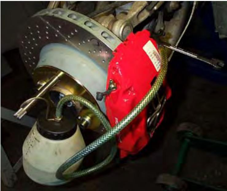
Have your assistant sit in the driver's seat and press the brake pedal on your command. After the brake pedal is depressed, open the bleeder screw quickly and then close it before the brake pedal sinks all the way to the floor. Repeat this a few times until there are no longer ANY air bubbles visible in the clear plastic hose.
