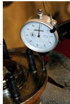
Measure runout at the rotor and bearing flange.
