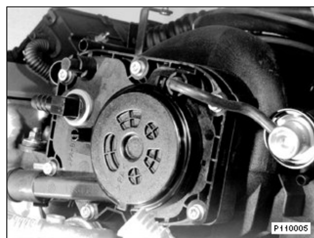
Pressure control valve in intake system
