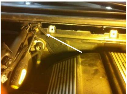
Remove firewall cover. There is a twist off clip on the driver corner and 2 torx screws that hold it n.
