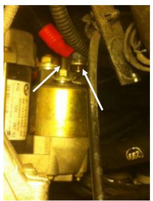
Disconnect electrical wires from starter, from top or bottom, whichever is easiest. Make sure to note where the 4 wires on the starter go.
