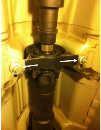
Once you unbolt the center support bearing, let it hang free and slide the front driveshaft back. Support it off to the side.
