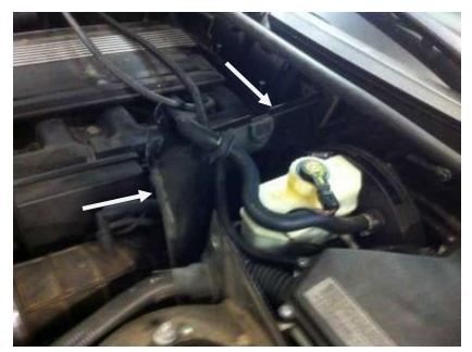
Remove cover next to ABS pump. Take off the weather stripping that is on top of this cover. That provides access to the 2 rubber grommets that hold the booster hose and wiring loom. Just slide those 2 grommets upwards and that will then free up the plastic cover-allowing you to remove it.
