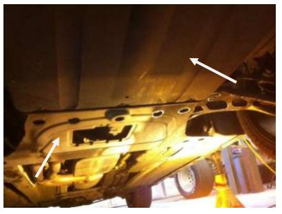
Remove plastic cover and front subframe cover. Plastic Cover is just Phillips screw driver The subframe cover has 8- 16MM bolts.
