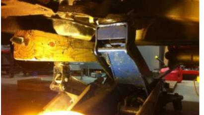
I added a second jack with a 4x4 spanning the trans pan for additional security.
