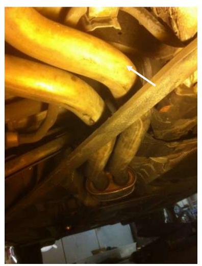
Remove the angled brace on the driver side that goes from near the rear jack point to a metal cover over the differential. Remove the 4 bolts and pull it out of the way.
