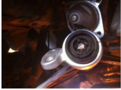
I would suggest threading the starter bolts into the new starter before installing it to ensure the threads match up okay. Mine were not perfect and I had to tap them to remove some paint that made the threads a bit thicker. Better to check the thread pattern with the starter in your hand then after you have worked it back onto the car.
