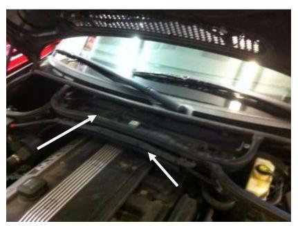
Remove cabin air filter housing. There are 3 twist off clips and then 4 torx screws at the back of the air filter housing. Unclip the positive cable that is attached to the front of the housing and you can then pull it out.
