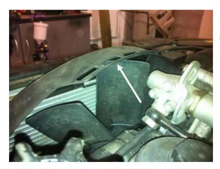
SLOWLY lower transmission until rear of cylinder head touches firewall. If auto tranny, only tilt engine until top of fan touches fan shroud. (Mine is auto trans). Since I used 2 jacks I had to lower both at the same time.
