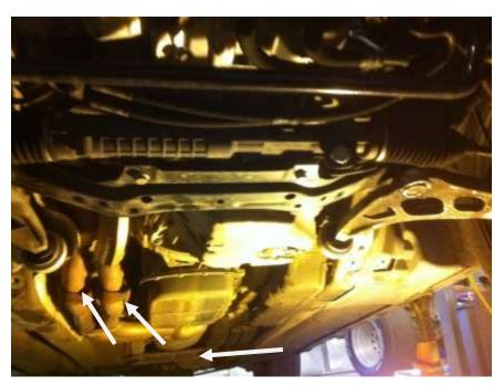
Remove exhaust. The exhaust is one long heavy piece. There are 4 nuts to remove at the end of the cat converters (see arrows in pic). It might be wise to spray with penetrating oil as these will likely be rusted tight. These nuts are copper, so they will round off easy, make sure you have the socket on the nut properly to reduce this risk. I think they are 15MM
