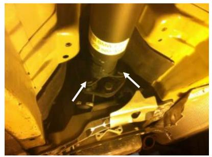
Disconnect the front of driveshaft from transmission. There are 3 bolts that go through the driveshaft into the guibo. 18MM ratchet on the bolt head and 18MM open end wrench on the nut. Leave the guibo attached to the trans.
