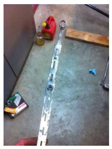
I unfortunately do not have a picture from the top side. I found it easier to remove the top starter bolt from the top of the engine.
