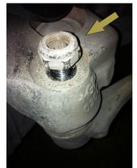
Step 5: Loosen 18mm nut on the bushing side of the arm with a breaker bar. You will need to hold the bolt side with a 16mm wrench or ratchet eventually but you might get away with at least loosening it with the breaker bar before you have to get in there with both hands. No need to remove the bolt completely at this point, it will be much easier once you have removed the ball joint.
