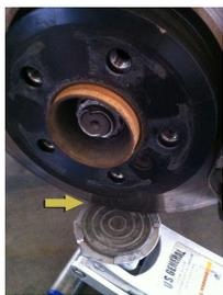
Step 9: By rotating the steering angle and a jacking up the assembly with a floor jack under the rotor, move the knuckle and ball joint around until you can get it to go back through the hole. Loosely attach the nut 22mm nut (this should be a new one also, plus you've probably creamed the old one so shouldn't have trouble telling which is new and which is old).
