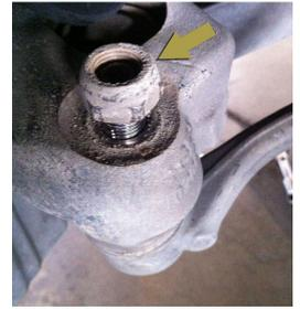
Step 7: Wiggle around the ball joint until it comes loose and let the control arm fall and hang on the bushing side bolt. Now the 16mm bolt at the bushing should be easy to take out, along with the control arm.
