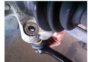
Step 10: Now go back and tighten the bolt/nut at the bushing side. I used my torque wrench set to 80 nm but that was kind of a guess (yikes). Can anyone confirm the correct torque here?
