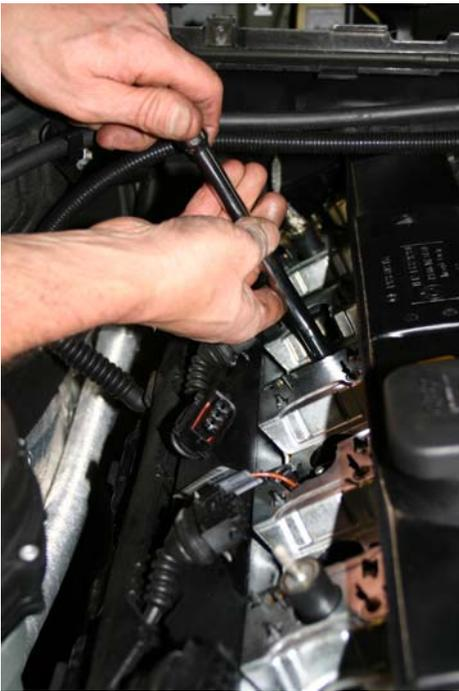
Replacing spark plugs in an M54 engine.
