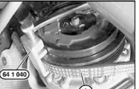
Crank engine at central bolt in direction of rotation until drive belt is fully guided in belt pulley.
