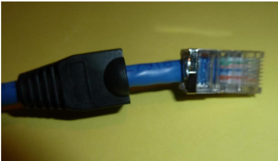
Here's the completed RJ-45. The brown wire is soldered to the shielded casing of the RJ-45 and ready to be covered by the connector boot.
