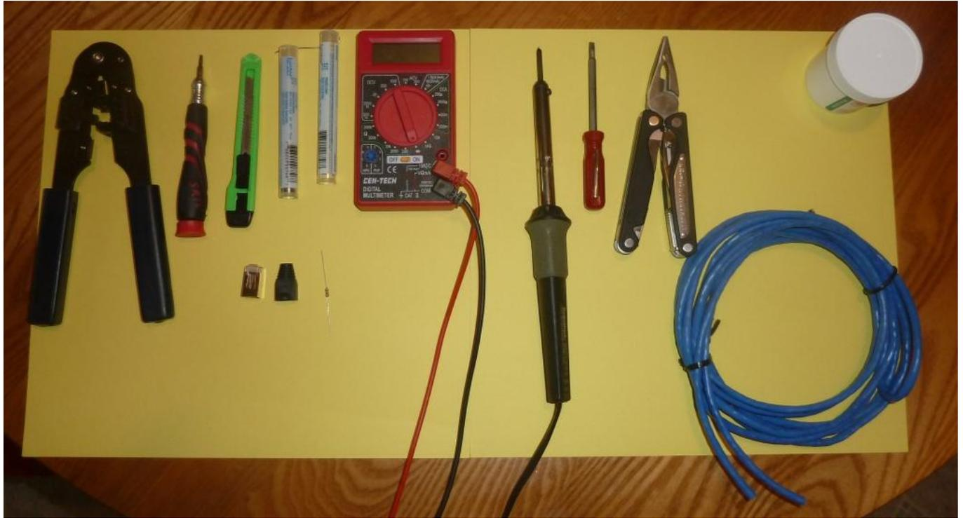
These are the tools I use to make my cables. The only specialty tool is the network cable crimper. I'm using a simple and cheap multimeter to show that you don't need anything special to test your cable. The only thing missing from the picture is the OBD2 connector.
