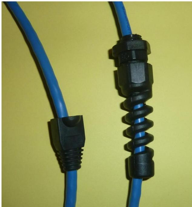
Next put on the RJ-45 boot and OBD2 connector cable protector. You don't want to crimp the RJ-45 or solder your OBD2 connector only to find out you forgot to put these on the cable first.
