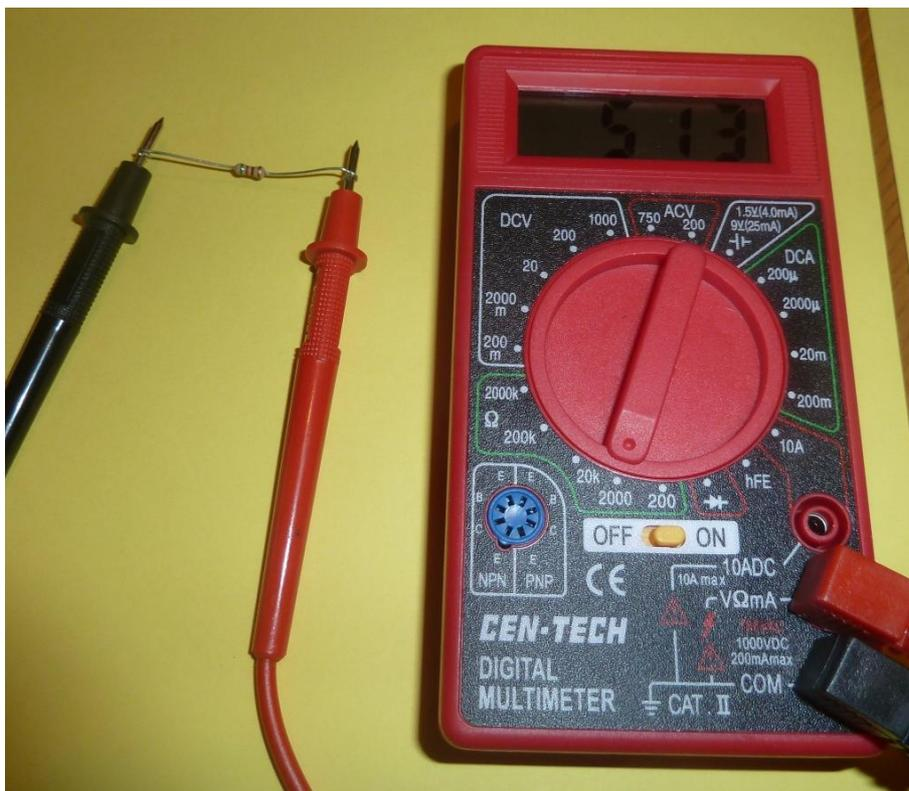
First I test the resistor to make sure it doesn't fluctuate all over the place. So long as it sits stable between 506 and 560 ohms you are set.
