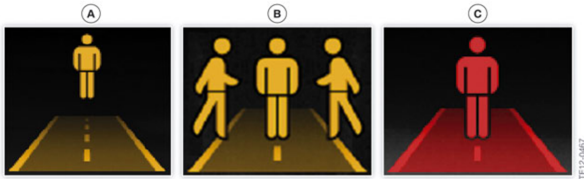
F01/F02 LCI - Pedestrian warning in the instrument cluster display or in the head-up display
