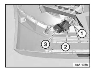
Unfasten plug connection (1) and disconnect. Release nut (2) and remove fanfare horn (3).
