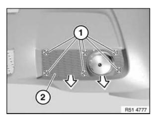
Release catches (1) on trim (2) with special tool 00 9 317 and remove trim (2).
