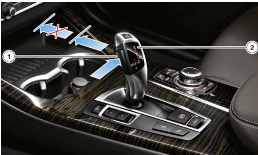
F25 Electronic transmission emergency release, GA8HP
