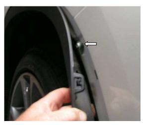
4. Remove 9x 8mm screws from the bottom edge of the fascia.
