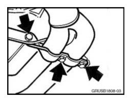
2. Remove the lower bracket for the exhaust system. If droning/vibration is gone, proceed to step three. If vibration/droning still exists with the lower bracket removed; continue troubleshooting exhaust/driveline for other causes or conditions
