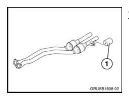
(1) with the 32hz dampener PN 18 10 7 506 145. Tighten to 21Nm.
