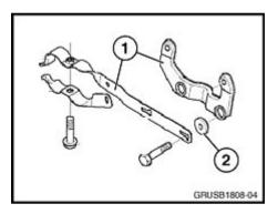
3. Remove complete bracket assembly and replace it with the bracket (1) PN 18 20 7 521 346 using two new ASA bolts (PN 07 12 9 905 417. Tighten to 21Nm.
