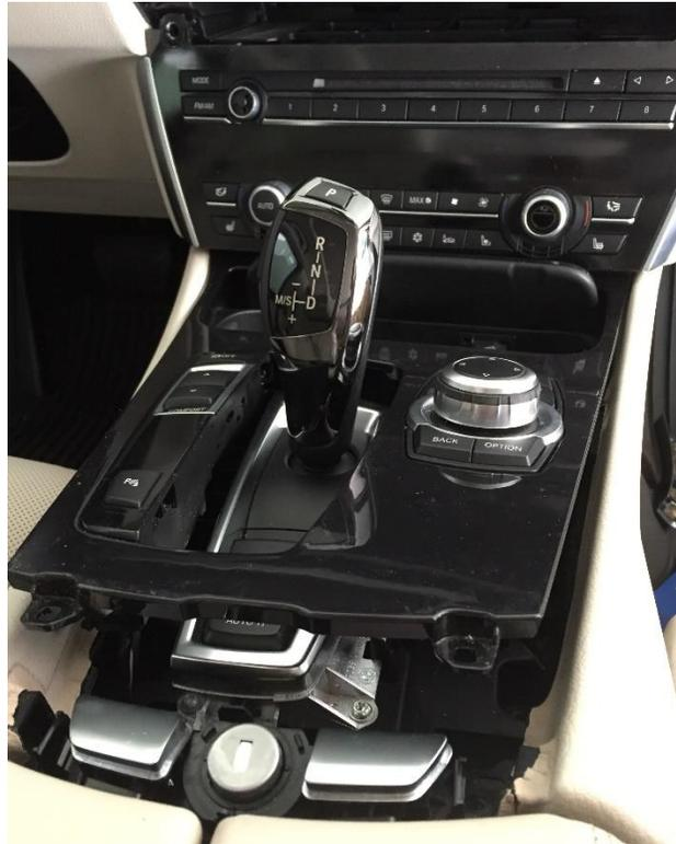
\*Note: The parking sensor electrical harness proved difficult for me as it was so small I couldn't gain leverage to remove. Instead I detached the cluster that contains both the parking sensor and driving mode buttons from underneath (see picture below for location). Using a 1/4" socket wrench worked best due to tight working space.
