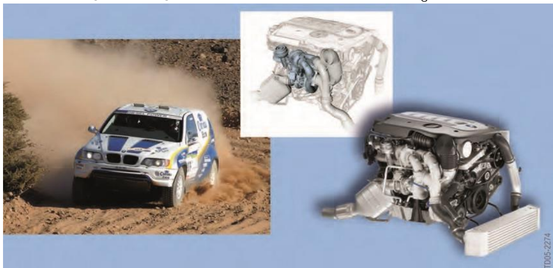
8 - BMW X5 3.0d with M57TU TOP engine in the 2-stage turbocharging system. The diesel engine in the
