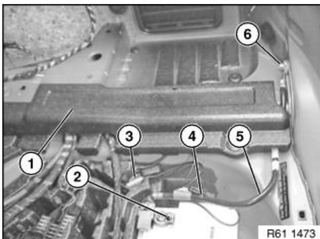
Remove underlay for floor panel (1).
