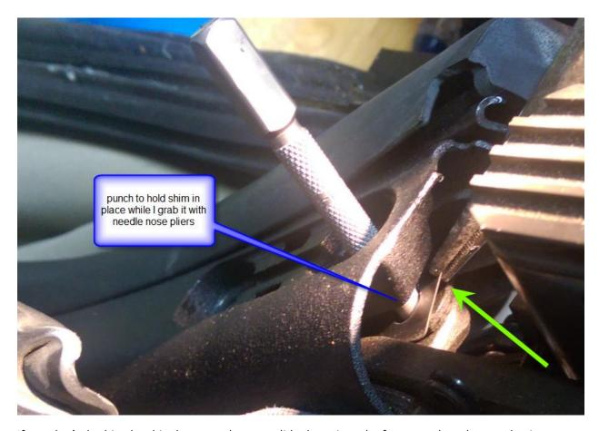
If you don't do this, the shim has a tendency to slide down into the frame, and can be a real pain to retrieve.
