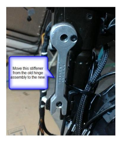
Note position of wires, and especially plastic zip ties. Take a few photos here, as you really don't want a hydraulic line or electrical wire to be in a pinch position after re-assembly.
