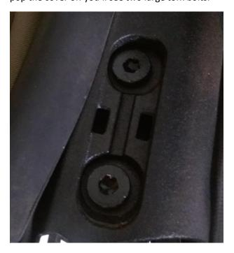
Remove the torx bolt that is further from the hydraulic cylinder first. Once it's out, place a punch or small screwdriver in the hole, and then remove the second bolt. The reason for the punch is that there is a small aluminum shim between the hinge parts and the frame. The punch will hold it in place till the hinge arms pull away from the top frame, and you can reach in and grab it with a pair of needle nose pliers.
