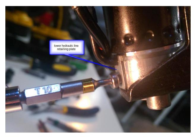
Once the retaining plate is out, pull the hydraulic line straight out. There is a stinger that is simply inserted into the cylinder about 3/8 of an inch. Place it directly into the new cylinder, and install the retaining plate and screw.
