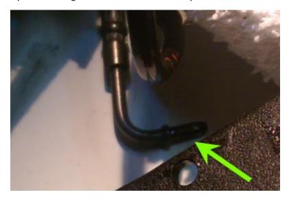
For the top line there is a small metal clip that is holding the stinger into the cylinder. You can simply push this off (away from the open end) with your thumbs. Once removed, the stinger will slide out just like the lower unit. Place it into the new cylinder and push the retaining clip back on.
