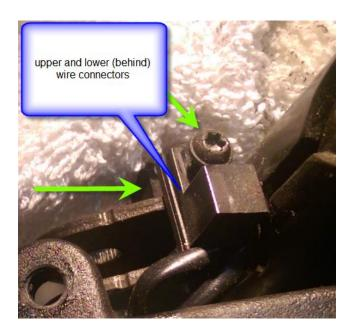
For re-assembly, line hinge pins back up and put the torx drive pin back in first. This helps alignment of the other pin.
