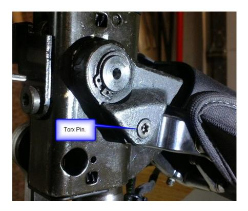
Pin two has a retaining ring on the back (inside) of the assembly. Remove the retaining ring using a small flat screwdriver. There is a slight recess on the opposite side of the ring from the opening. Place a small flat screwdriver into the recess, twist slightly and the ring will pop off the pin in perfect condition. Save, as you will re-use these pieces.
